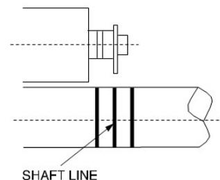
In case the coupling is used, it may be considered that the rotor can be easily moved in the axial direction. In fact, however, it hardly slides in the axial direction at the coupling as the torque grows greater. When by some reason the rotor has undergone some axial movement, and the coupling does not provide enough slip to allow the rotor to return to the magnetic center of the motor, it will continue to operate with the bearing end in contact with the shoulder of the journal.
